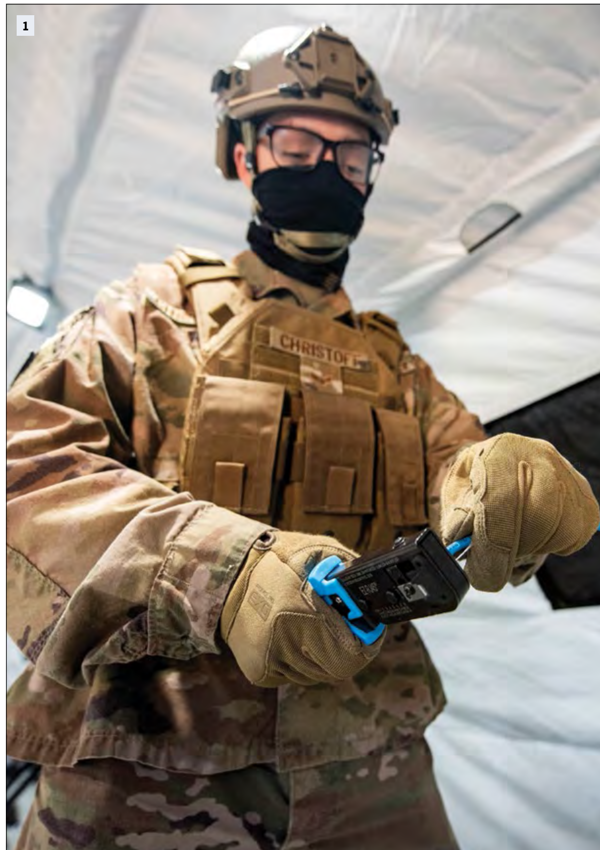
1) U.S. Air Force Airman 1st Class Stone Christoff, 821st Contingency Response Support Squadron, uses a crimping tool to finish building a CAT5 cable during a "Crow's Nest" exercise April 30 near the Global Reach Deployment Center on Travis Air Force Base, California. Christoff built several CAT5 cables in order to wire the tent for future connectivity.
